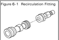
Attach one section of female/female solution hose to the outgoing solution fitting on the front of the machine and the other end to the garden hose and recirculation fitting combination that is attached to the front of the machine(or as many sections as you want, if you wish to freeze guard your hoses).
