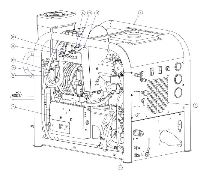
Figure 9-4 Machine Assembly - Rear View - Left Side
